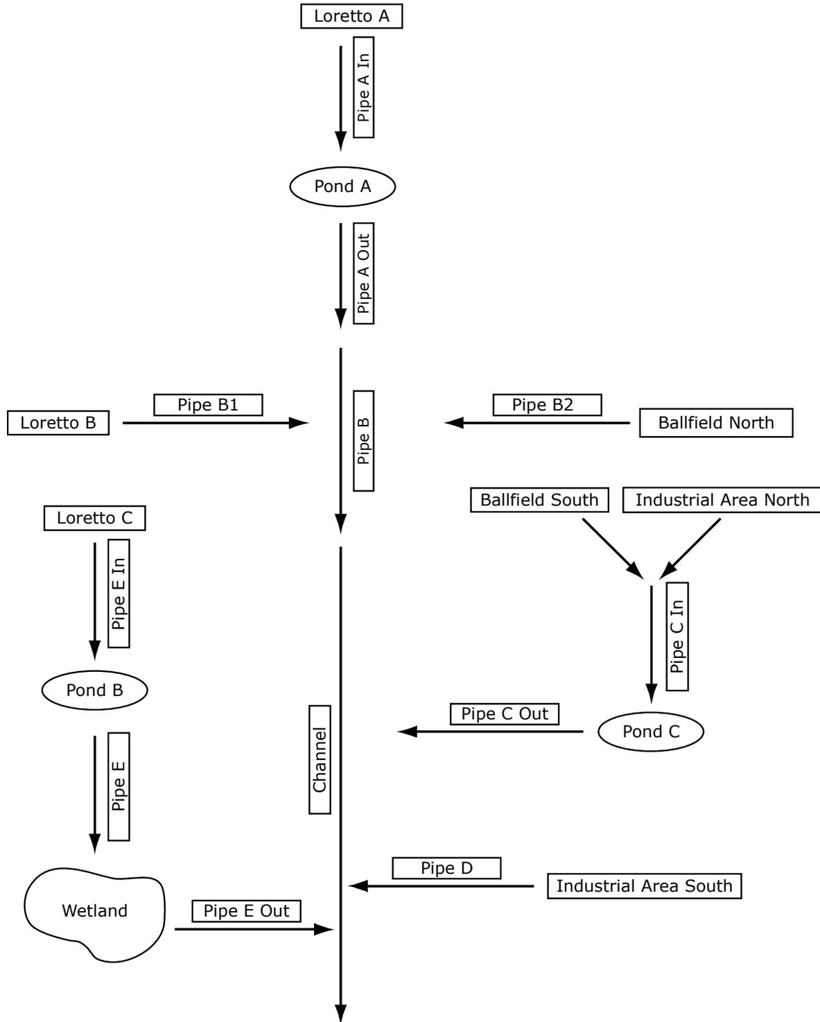
Figure 3.3. Conceptual flow diagram for the P8 model of Loretto.
