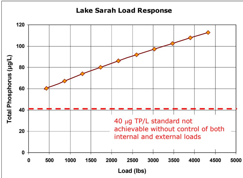
**Figure 4.1.** Lake Sarah load-response with an internal loading rate of 1.0 mg/m<sup>2</sup>/day and 10-year average watershed loading in the BATHTUB model.
